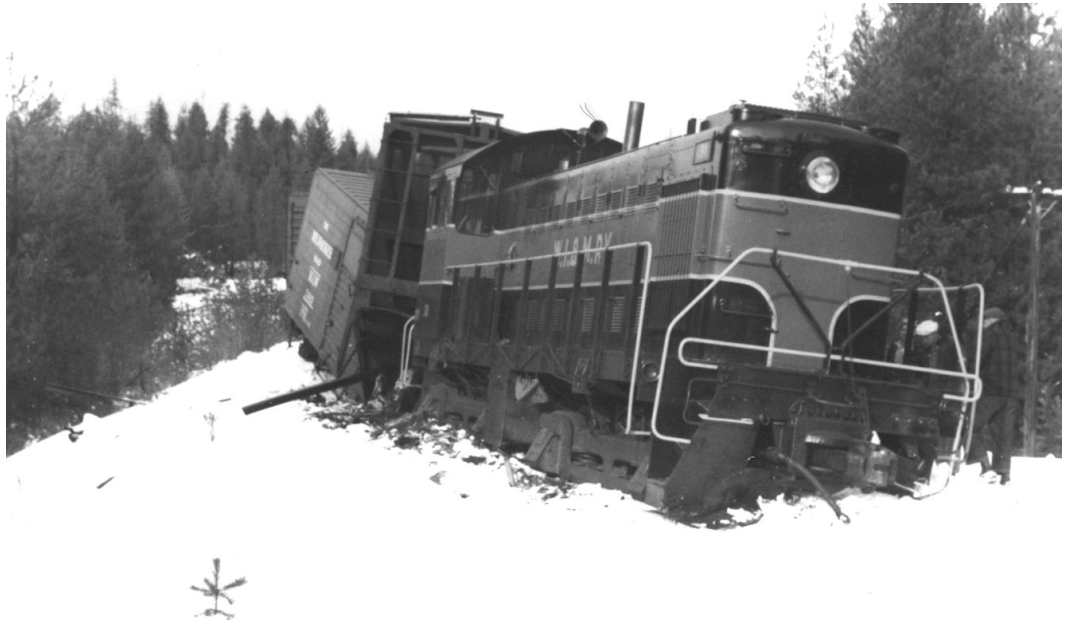
WI&M locomotive #30 has sunk to its axles in muddy snow after a fill washed out under the weight of its train in February, 1965. Photo: University of Idaho Special Collections Library
