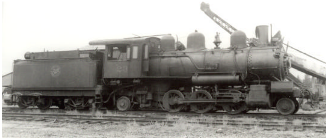
Locomotive number 23 takes a break at the Potlatch Lumber Co.'s shops north of Bovill. This engine spent most of its career in this area, bringing long trains of logs out of the mountains. By the time this photo was taken in 1947, #23 had been converted from burning wood to burning oil. Even at this late date, the little Prairie still had a few years of work ahead. Tom Burg Collection
