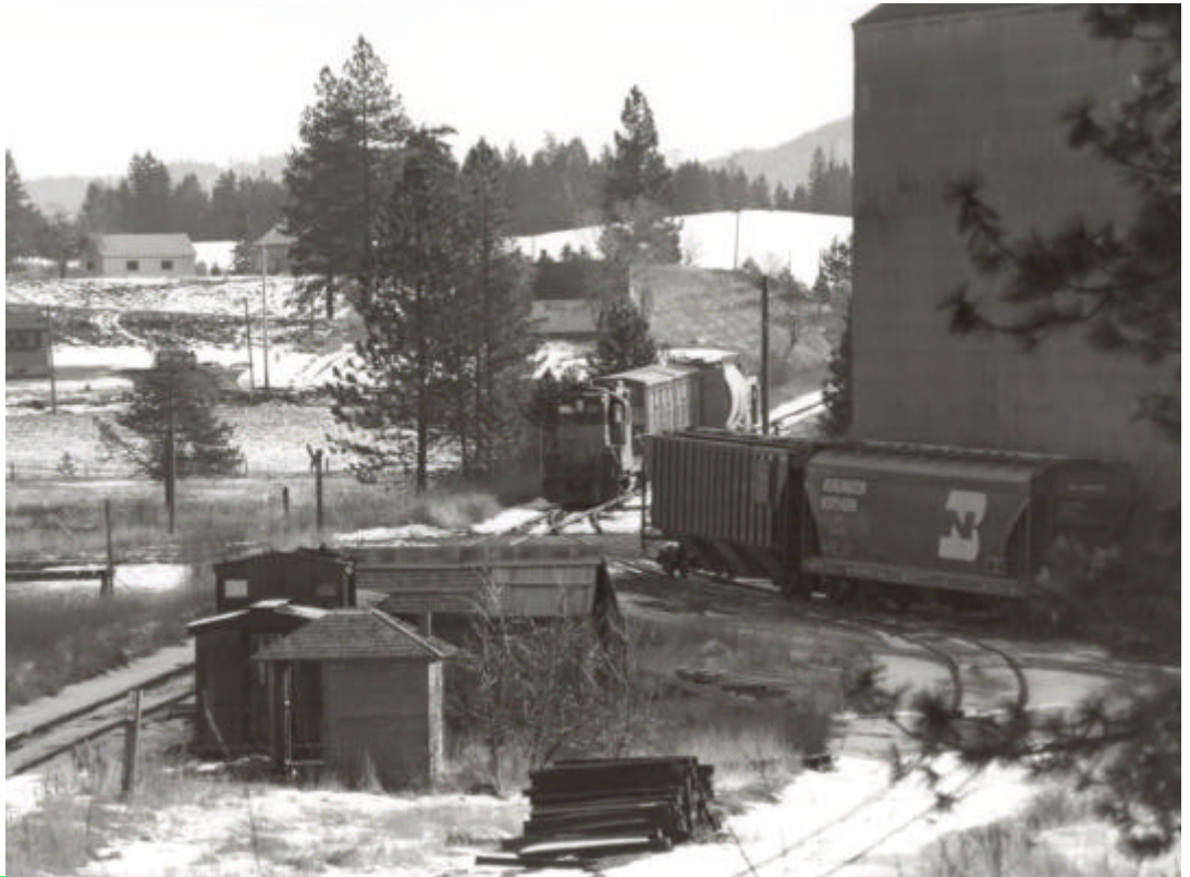
This January 1977 view of a short WI&M train behind Milwaukee Road GP-9 287, shows all the classic railroad elements of Deary still in place. Caboose X-1, now on blocks, serves as a replacement for the original depot, but the privy and section house remain. Two 100-ton grain hoppers sit on the elevator spur, awaiting pickup by a later train. Carl Sonner Photo
